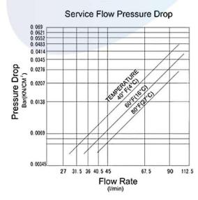
The difference in pressure between two points in a system, caused by resistance to flow. Pressure drop is pressure loss across the valve created by system demand - not by the valve alone.
